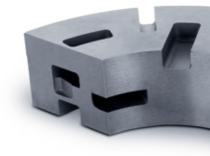
Cemented carbide is a sintered material that is primarily manufactured from **tungsten carbide** and a binding agent—usually cobalt. **A low binding agent content increases the wear resistance—a higher content the toughness.** The selection of the grain size influences the following properties:
